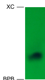
Figure 4. Electrophoresis of the heptamer [d(C PS 2 T PS 2 G PS 2 A PS 2 C PS 2 T PS 2 T)] on a 20% polyacrylamide gel containing 7 M urea, visualized by UV-shadowing.
